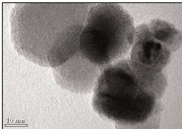
QSI-Nano® iron is available in sizes ranging from 10 to 40 nanometers. Iron content is controlled by oxide thickness and can range from 30% wt. to 50% wt.
