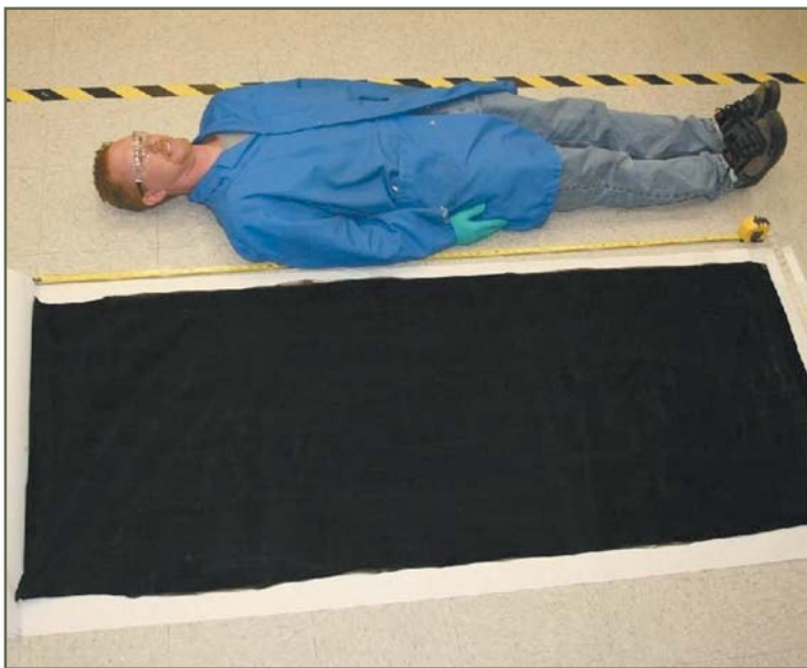
Nanocomp Technologies recently announced that they have manufactured the largest cohesive sheet of nanotube material ever in 3' by 6' sheets.
